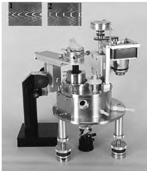
**Fig. 2.** Photographic image of the surface forces apparatus Mark IV and images of FECO fringes when the mica surfaces are close to contact (1), and when they are in adhesive contact (2). Figure adapted from <http://www.rsphysse.anu.edu.au/SFA/>, with permission. From the Australian National University, Tim Wetherell.
