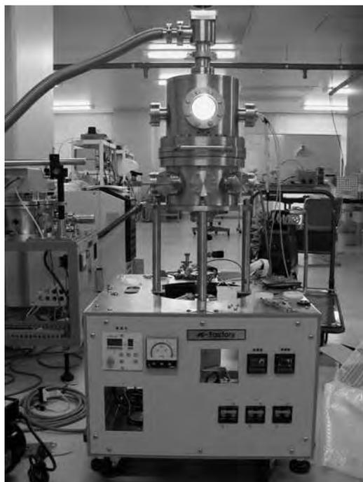
**Fig. 11.** Photo of the CVD apparatus for the large size substrates.
