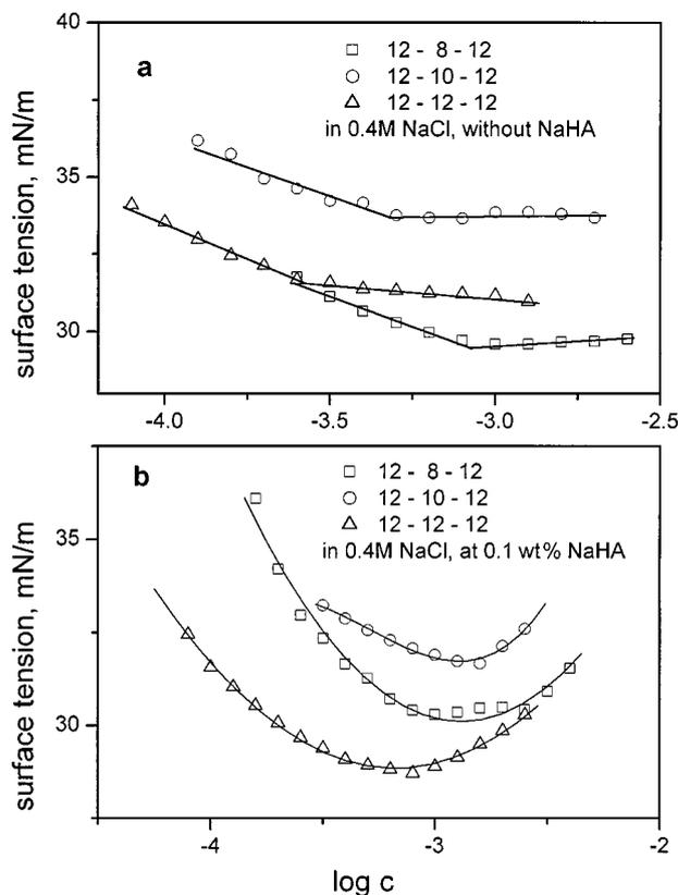
**FIG. 1.** Surface tension of NaCl–12- $s$ -12 dimeric surfactant system in aqueous 0.40 M NaCl solution vs  $\log c$  at different surfactant structures (variable parameter  $s$ ). (a) Without NaHA. (b) With 0.1 wt% NaHA.
