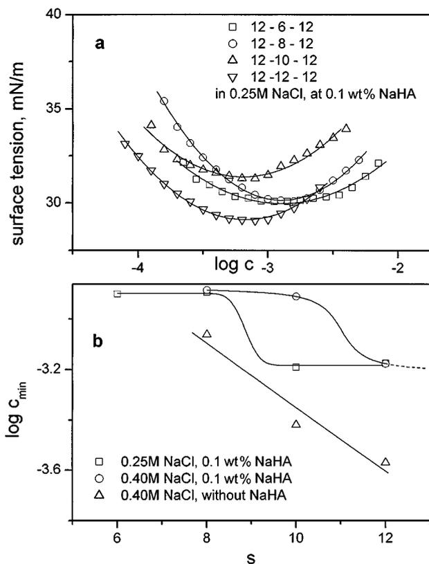
**FIG. 2.** (a) Surface tension of 0.1 wt% NaHA-NaCl-12-*s*-12 dimeric surfactant system in aqueous 0.25 M NaCl solution vs  $\log c$  at different surfactant structures (variable parameter  $s$ ). (b) Plot of  $\log c_{\min}$  obtained from Figs. 1b and 2a vs parameter  $s$ . The cmc of 0.40 M NaCl-12-*s*-12 dimeric surfactant system without NaHA is included as symbol  $\Delta$ .
