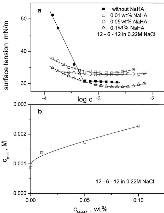
**FIG. 3.** (a) Surface tension of NaHA-NaCl-12-*s*-12 dimeric surfactant system in aqueous 0.22 M NaCl solution vs  $\log c$  at different NaHA concentration  $c_{\text{NaHA}}$ . (b) Plot of surfactant concentration at minimum viscosity  $c_{\min}$  obtained from Fig. 3a vs  $c_{\text{NaHA}}$ .
