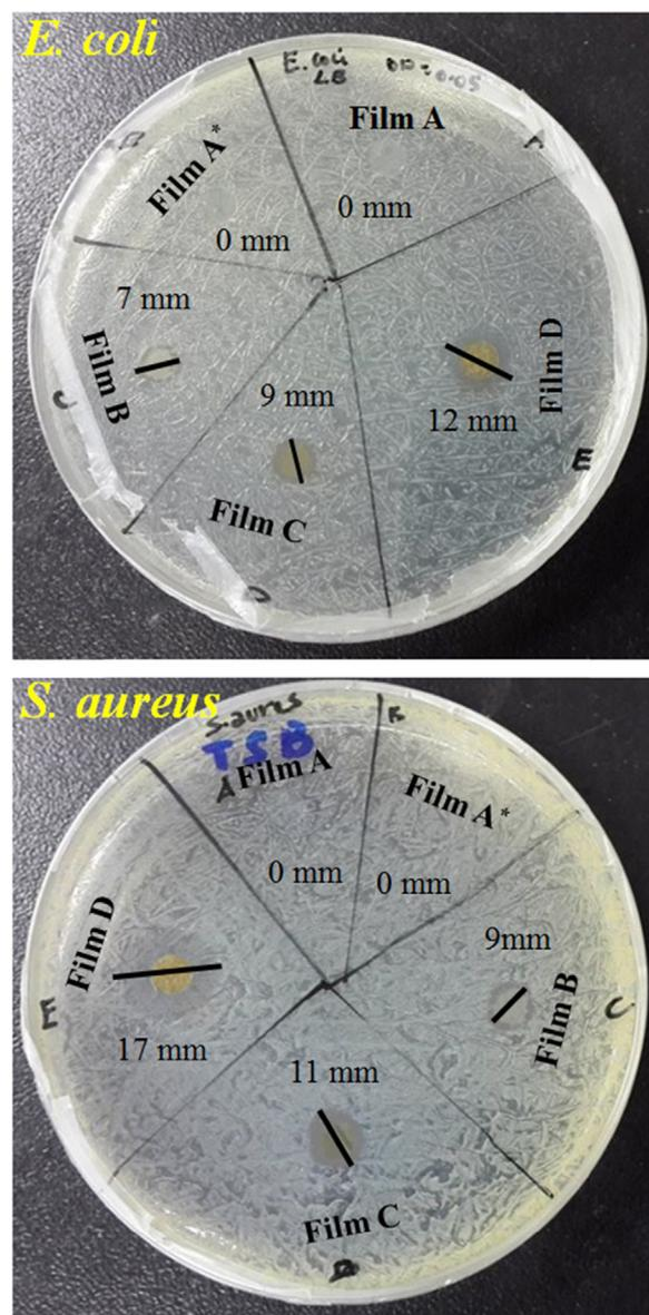
**Fig. 8.** Antibacterial activity of NFC (Film A), DEN-NFC (Film A\*) and DENAgNPs-NFC (Film B–D) films against *Escherichia coli* and *Staphylococcus aureus*.
