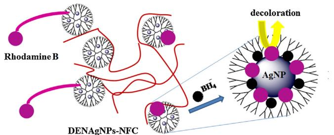
**Fig. 7.** Schematic mechanism of decoloration of Rhodamine B by NaBH<sub>4</sub> in the presence of DENAgNPs-NFC film.
