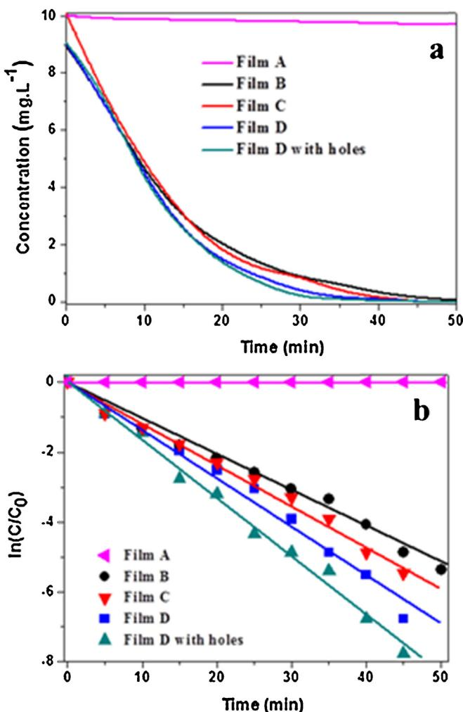
**Fig. 6.** (a) Curves of Rhodamine B concentration versus reaction time and (b) decay kinetics profiles of Rhodamine B in existence of NFC (Film A) and DENAgNPs-NFC (Film B-D) films (calculated from Fig. S6 in Appendix A).
