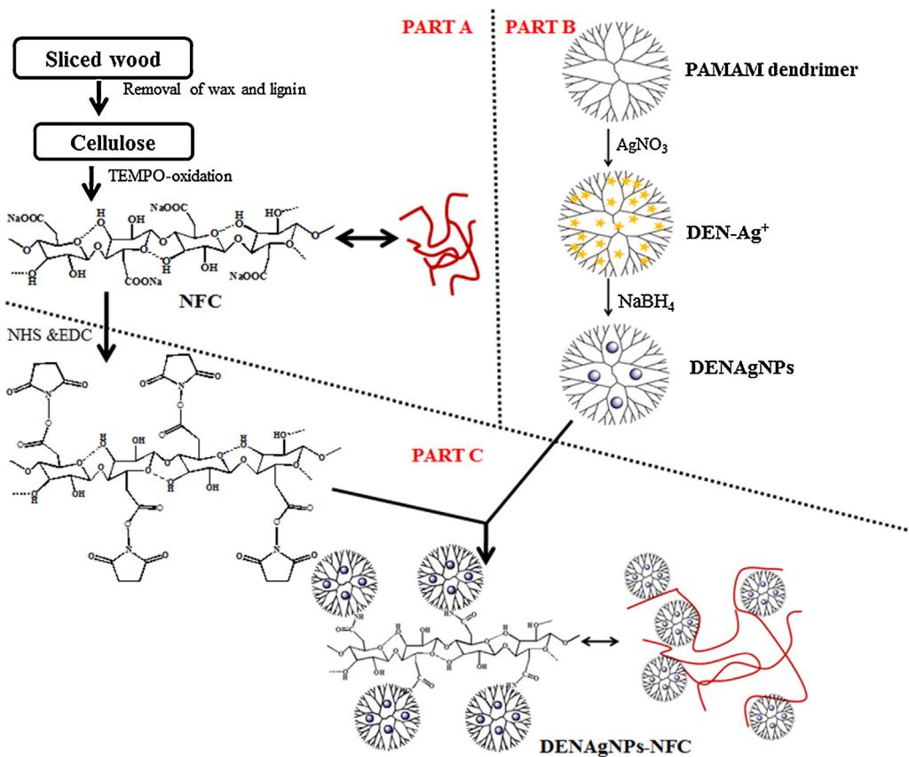
**Fig. 1.** Schematic illustration of amidation reaction between NFC and DENAgNPs.
