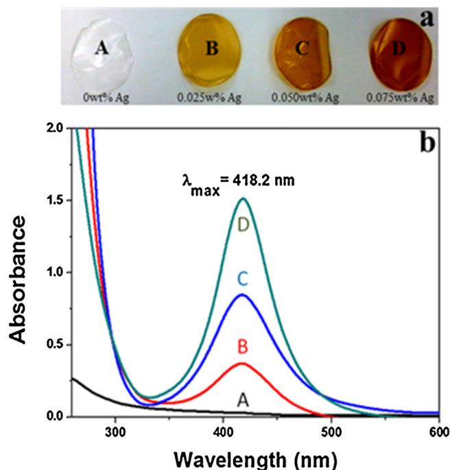
Fig. 2. (a) Visual observation and (b) UV-visible absorption spectra of NFC (A) and DENAgNPs-NFC (B–D) films.
