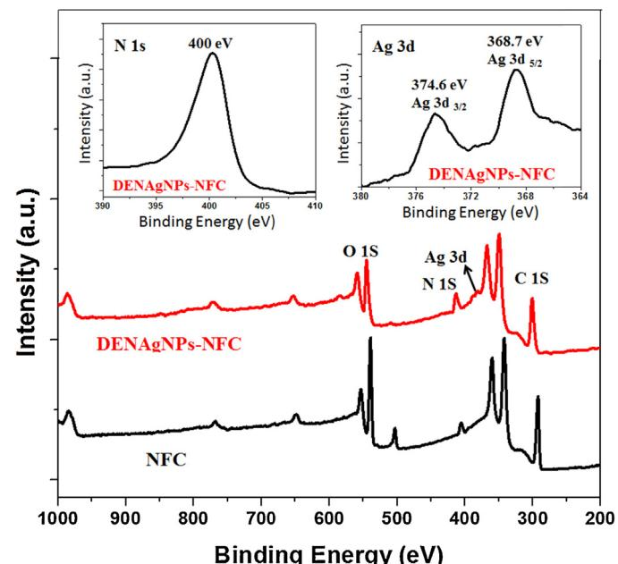
**Fig. 5.** XPS of NFC (Film A) and DENAgNPs-NFC (Film B) films.
