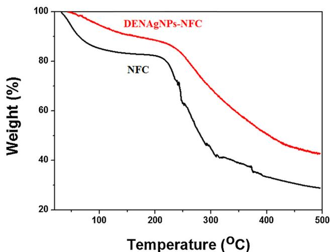
Fig. 4. Variation of mass with temperature during the thermogravimetric analysis of NFC (Film A) and DENAgNPs-NFC (Film B) films.
