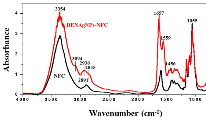
**Fig. 3.** FT-IR absorption spectra of NFC (Film A) and DENAgNPs-NFC (Film B) films.
