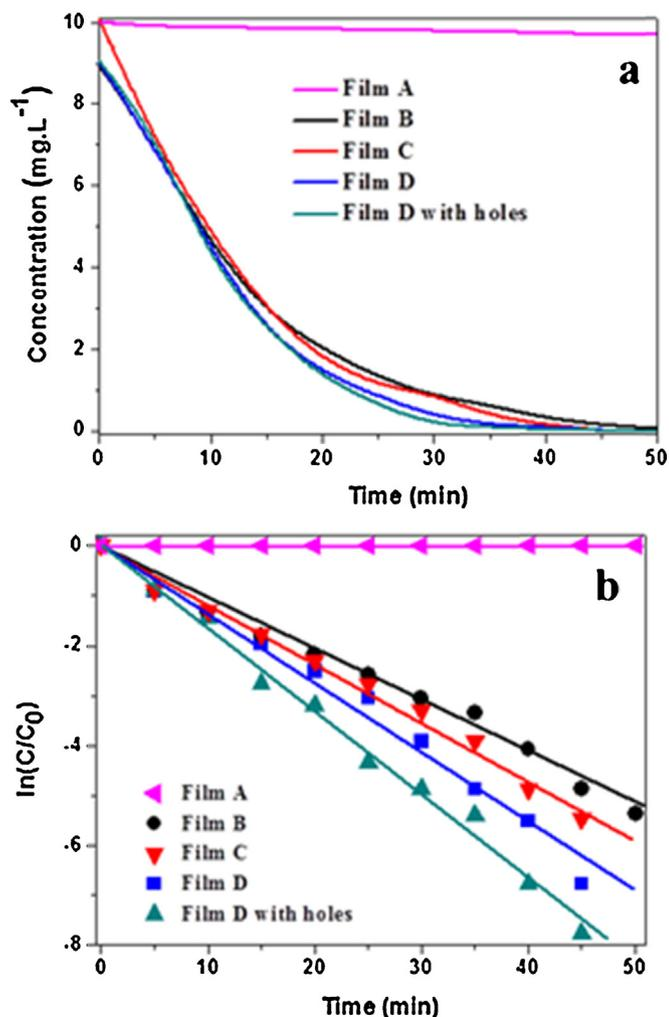
**Fig. 6.** (a) Curves of Rhodamine B concentration versus reaction time and (b) decay kinetics profiles of Rhodamine B in existence of NFC (Film A) and DENAgNPs-NFC (Film B–D) films (calculated from Fig. S6 in Appendix A).
