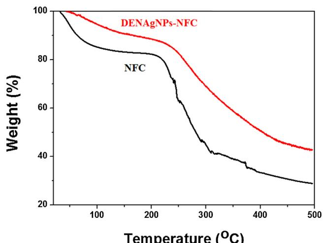
**Fig. 4.** Variation of mass with temperature during the thermogravimetric analysis of NFC (Film A) and DENAgNPs-NFC (Film B) films.
