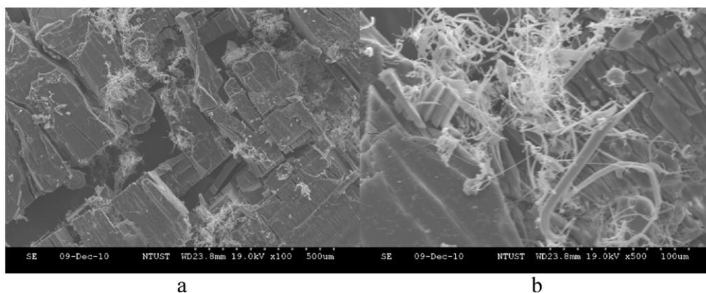
**Fig. 6.** SEM micrograph of PLLA surface immersing in the human gastric juice for 42 days. (a) Crack region (b) fiber-like region.
