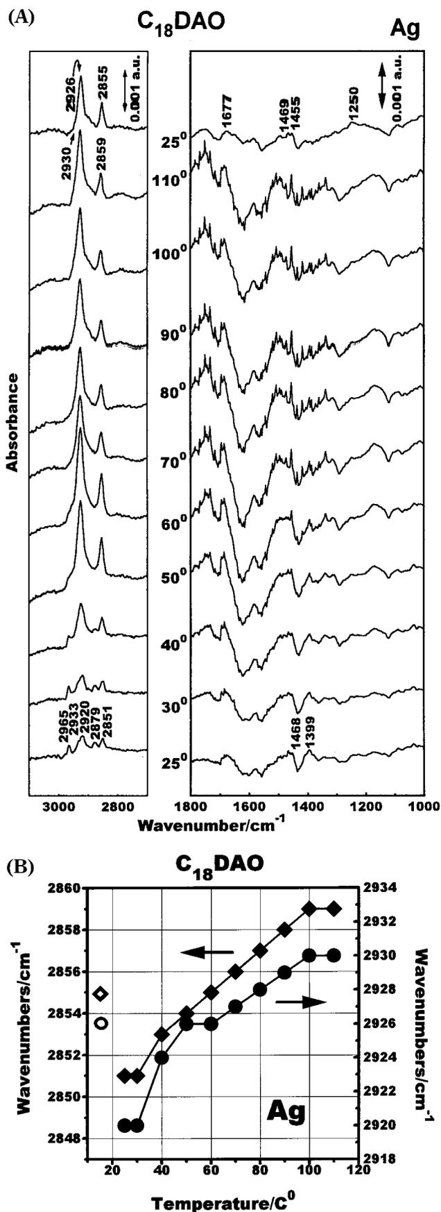
**Figure 5.** (A) Temperature-dependent changes in an IR RA spectrum of five-monolayer LB film of  $C_{18}DAO$  on a silver-evaporated glass slide. (B) Temperature dependences of the frequencies of the  $CH_2$  stretching bands for the spectra shown in (A).
