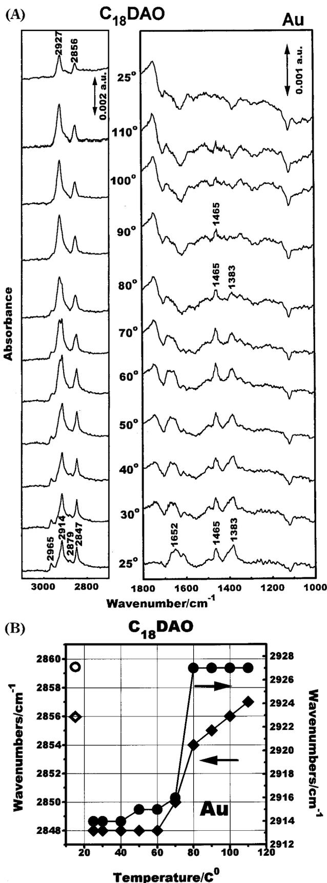
**Figure 1.** (A) Temperature-dependent changes in an IR RA spectrum of one-monolayer LB film of  $C_{18}DAO$  on a gold-evaporated glass slide. (B) Temperature dependences of the frequencies of the  $CH_2$  stretching bands for the spectra shown in (A). Throughout this paper the frequencies for the annealing films are presented by open circles (○) and squares (◇).
