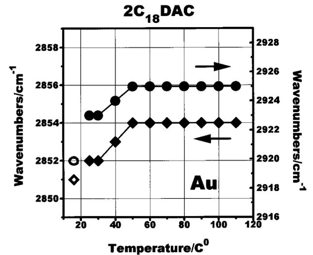
**Figure 3.** (A) Temperature-dependent changes in an IR RA spectrum of a five-monolayer LB film of  $C_{18}DAO$  on a gold-evaporated glass slide. (B) Temperature dependences of the frequencies of the  $CH_2$  stretching bands for the spectra shown in (A).
