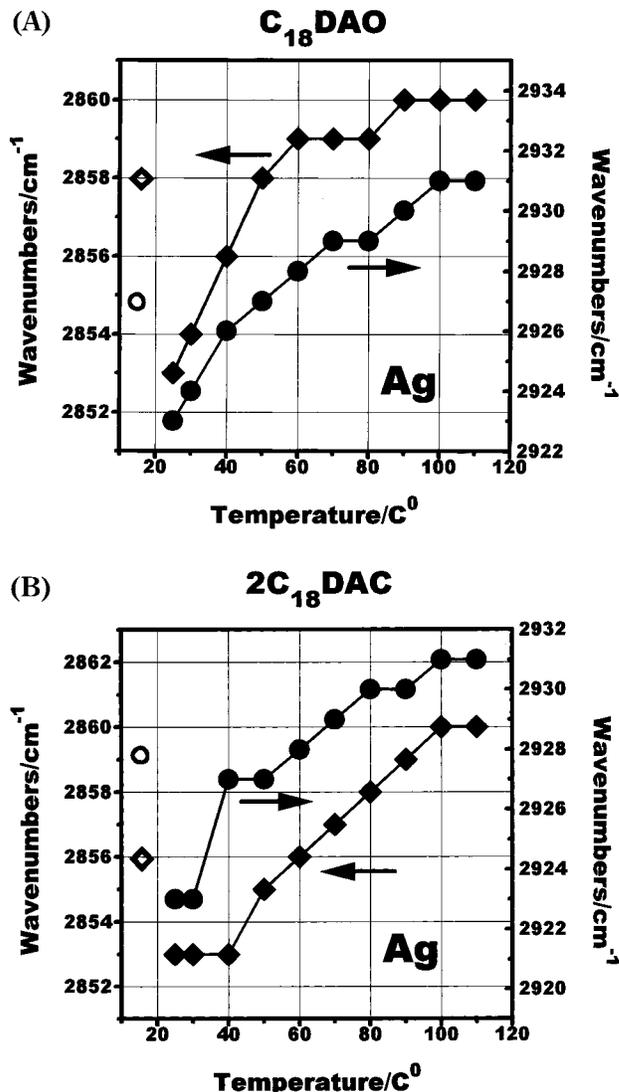
**Figure 7.** Temperature dependences of the frequencies of the  $CH_2$  stretching bands for one-monolayer LB films of  $C_{18}DAO$  (A) and  $2C_{18}DAC$  (B) on silver-evaporated glass slides.
