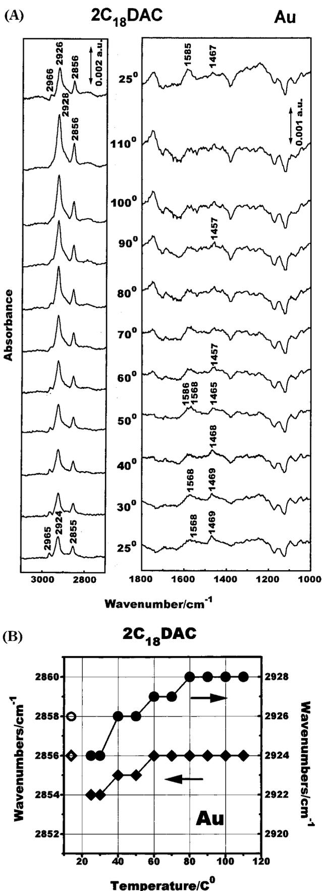
**Figure 2.** (A) Temperature-dependent changes in an IR RA spectrum of one-monolayer LB film of  $2C_{18}$ -DAC on a gold-evaporated glass slide. (B) Temperature dependences of the frequencies of the  $CH_2$  stretching bands for the spectra shown in (A).
