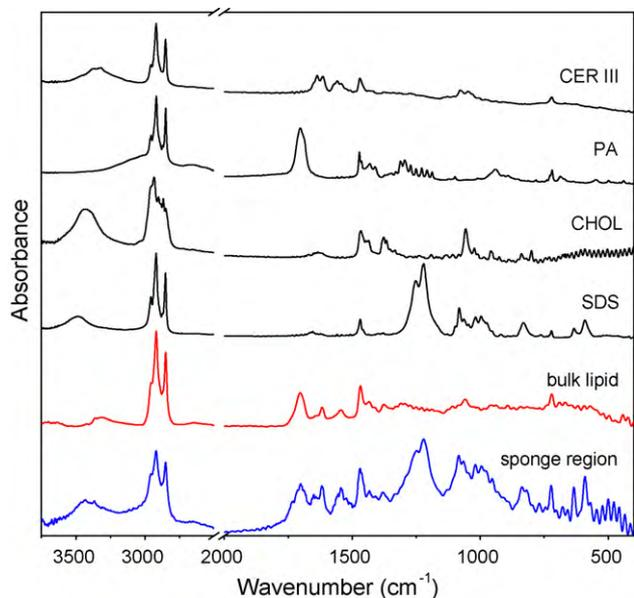
**Fig. 3.** Infrared absorption spectra of lipid membranes after exposed on an aqueous 10% SDS solution in comparison with component lipids.
