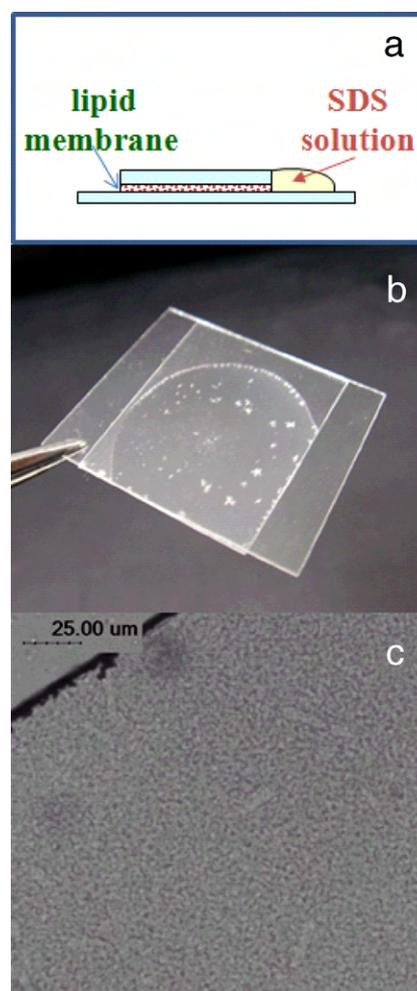
**Fig. 1.** A cartoon (a) and a photograph (b) of lipid membrane sandwiched between plates, and an optical microscopic image (c) of the membrane.
