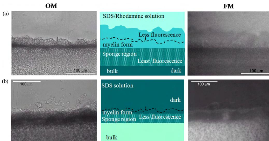
**Fig. 4.** Optical and fluorescence microscopic images of lipid membranes after exposed on an aqueous 10% SDS solution. (a) Rhodamine was solved in an SDS solution; (b) pyrene was mixed in lipid membrane.
