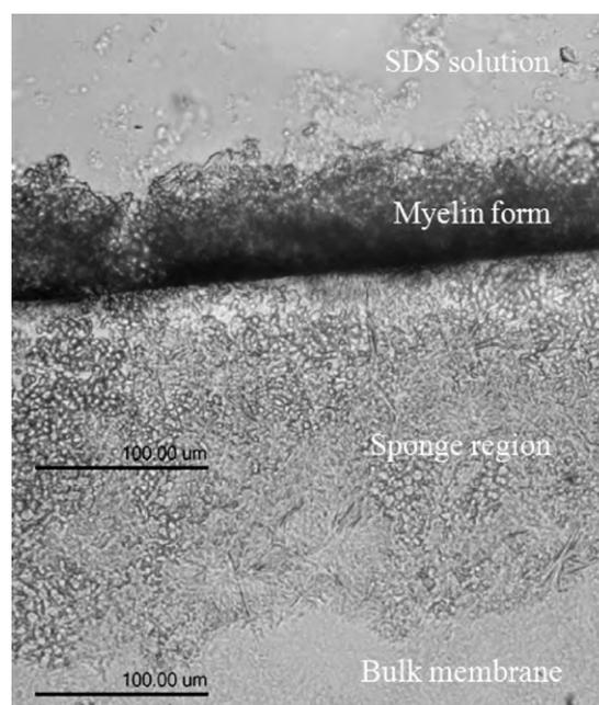
**Fig. 2.** An optical microscopic image of membrane of lipid mixture after exposed on an aqueous 10% SDS solution.
