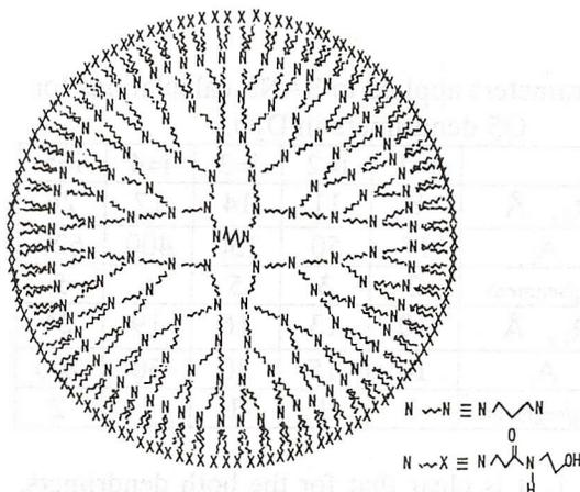
Fig. 1 Chemical structure of G5 PTMIN dendrimer with OH end groups.
