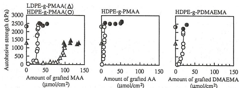
**Figure 3** Changes in the tensile shear adhesive strength with the grafted amount for grafted LDPE and HDPE plates.
